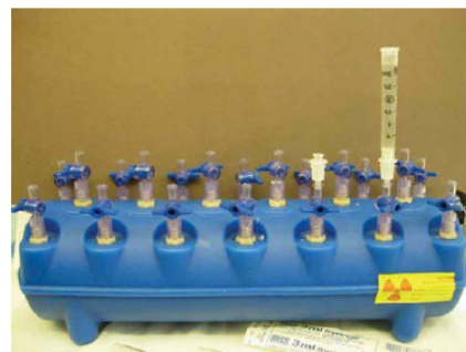
Figure 3 | Illustration of mini-scale purification using a vacuum manifold.
